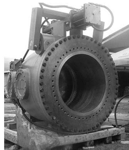
A 54-inch-diameter Pratt in-line Model 711 sleeve valve serves as a turbine bypass at the 12-MW Santa Ana hydropower plant in Bogotá, Colombia, part of an overall water supply project.
