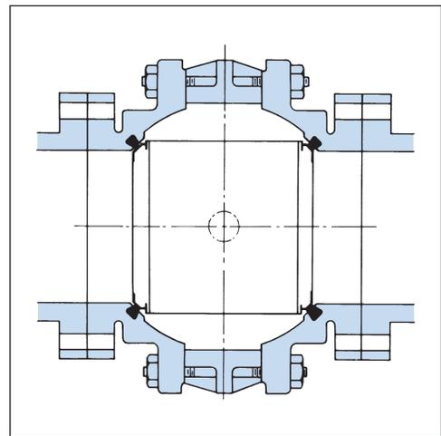
The cross-section drawing (above) illustrates the closed position utilizing dual seats.
