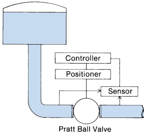
at any point from 15 to 75 psig. The non-electric system includes a pilot pressure operated three-way valve and a four-way valve and ball valve operating cylinder. Closing speed is adjustable. A dual supply pressure source with filter and check valves assures proper operating pressure for the control system. An electrical Set Point Control system that uses pressure switches as sensors will activate the valve with either a motor or water cylinder actuator.
