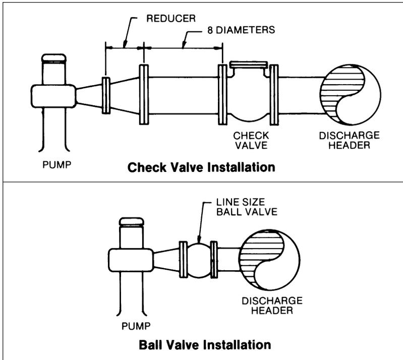
Center post and swing check valves have limitations based on maximum/minimum velocity and turbulence while efficient pump design has high exit velocities and considerable turbulence. The designer, therefore, must use an increaser on the pump discharge nozzle or specify a large discharge nozzle to accommodate the check valve. Additionally, some types of check valves require approximately 8 diameters of unrestricted pipe on the inlet side to ensure proper operation.
