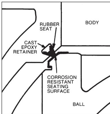
The E-LOK® seat design can assure longer seat life and better sealing action. By mounting the rubber seat in the body rather than on the ball the rubber seat is less likely to be damaged by debris in the flow stream where the valve is used in waste water applications.
