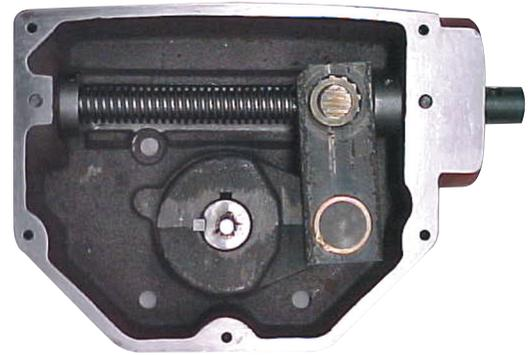
The Pratt MDT actuator is self-locking without a unidirectional sustained force from the valve. It can be relied upon to maintain exact valve position under conditions of fluctuating, turbulent and intermittent flow, yet one person can smoothly and easily operate the valve against full line pressure.
