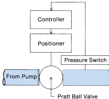
Controller output may operate the Pratt Positioner that utilizes water pressure as the operating medium.
