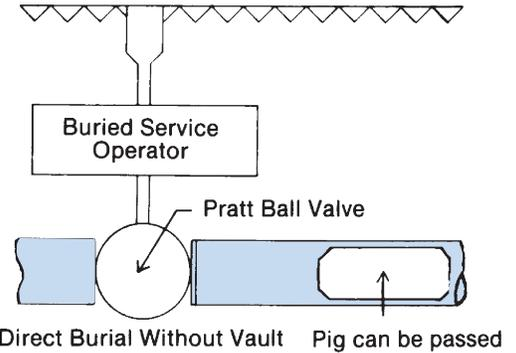
complete because the only contact between the body and ball is the rubber seat. The valve can remain in one position for years and still provide quick, reliable action when required. In underground lines, the valve may be directly buried without expensive concrete vaults.
