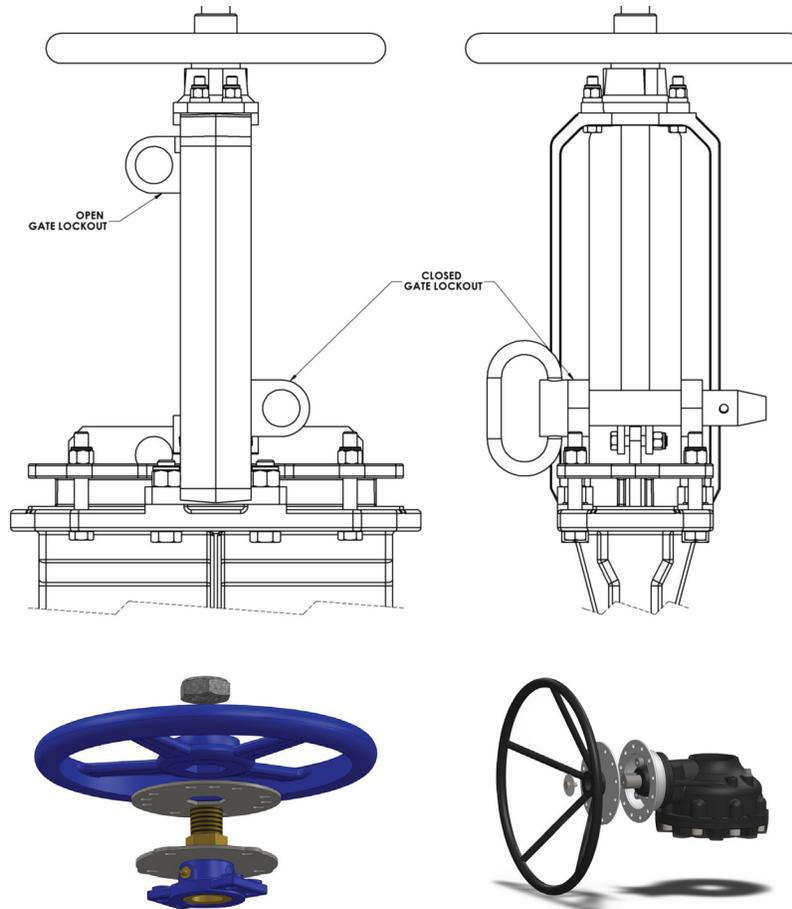
Gate lockout packages are available as open or closed only, or both open and closed.
