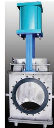
24" Figure 92 metal seat knife gate for throttling in oil sands. Tungsten carbide overlay on gate face, ID, and port ID.
