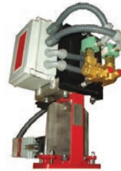
Double acting air cylinder, dual solenoid valve, and NAMCO limit switches wired to a NEMA 4 electrical box.
