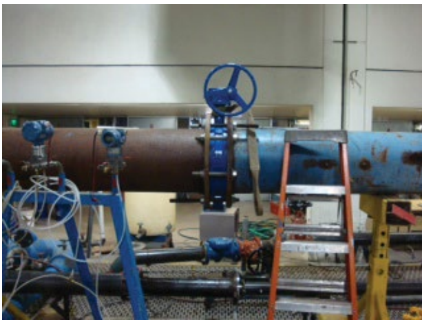
Pratt BF Series Wafer / Lug Butterfly Valves being tested at an independent research laboratory
