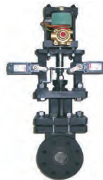
Figure F176, with air cylinders, open and closed position limit switches, and solenoid control valves. 310 SS for high temperature service.
