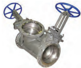
Custom fabricated 12" Figure 76 metal seated "modified Y" knife gate valve.
