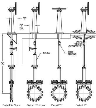
Detail 'A' Non- Detail 'B' No Rising Stem Rising Stem Offset Floorstand Floorstand Assembly Assembly
