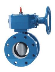
The Pratt® 2FII rubber seated butterfly valve is available in sizes 3" through 20". The shafts are constructed of centerless, ground ASTM A276 type 304 or 316 stainless steel bar and thus are not susceptible to corrosion as are carbon steel or other similar materials. Shafts are one-piece, through-shaft construction, sized to meet
