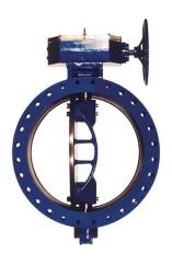
The Pratt® Triton® Butterfly Valve has a rubber seat located in the body that reduces performance problems related to corrosive buildup in valve body and pipeline. The E-Lok® seat can be adjusted and/or repaired in the field without dewatering the pipeline or removing the valve from the line. The flow through disc design allows more strength, less weight, and greater free flow area. Higher Cv: lower head loss results in
