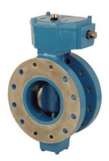
Pratt now offers a 350 psi, 525 shell test, ANSI 250#, Butterfly Valve – the first in the industry! This valve is excellent in high pressure applications. The valve body and disc are made of ductile iron with the rubber seat in the body for abrasion resistance and bubble-tight closure. Available in 6" – 48" with flanged end connections.
