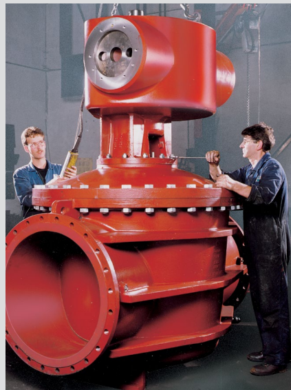
48" ROTARY CONE VALVE IN ASSEMBLY
